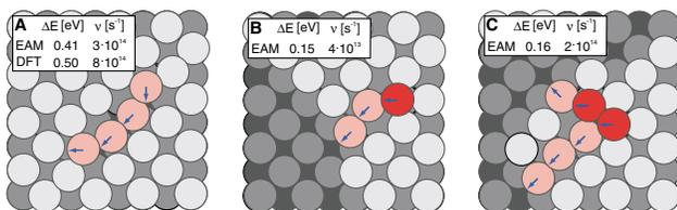
FIG. 1 (color). Multiatom processes seen in aluminum crystal growth simulations at 80 K include the four-atom concerted displacement process (a). The most commonly observed adatom descent process (b) also involves concerted displacement of several atoms. More than 20% of the activated processes involved three or more atoms such as the six atom concerted descent process shown in (c).
