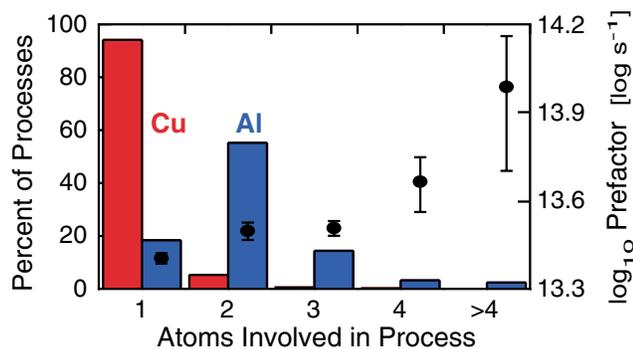
FIG. 4 (color). Most surface transitions observed in simulations of aluminum growth at 80 K involve two or more atoms, while single atom processes are most common in Cu. The transition rate has a larger prefactor, i.e., more favorable entropy contribution, when more atoms are involved in the process (see filled circles and the vertical axis to the right).
