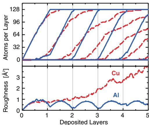
FIG. 2 (color). The upper panel shows the number of atoms in each deposited layer; the lower panel gives roughness [26].
