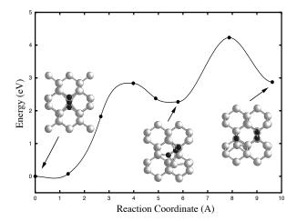
Figure 1: The minimum energy path for direct breakup of a  $B_3I^-$  cluster in silicon. The energy minimum far to the left corresponds to the nearly linear configuration of the three boron atoms. the minimum to the right corresponds to a boron dimer and a separate boron interstitial. The activation energy barrier for the break-up is high, 4.3 eV. The product  $B_2^{2-}$  is energetically unstable with respect to further break-up into individual  $B^-$  atoms at sites in the silicon lattice.
